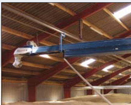
Kongskilde BCA belt conveyor - ideal for self-cleaning horizontal conveying where the space is narrow.
