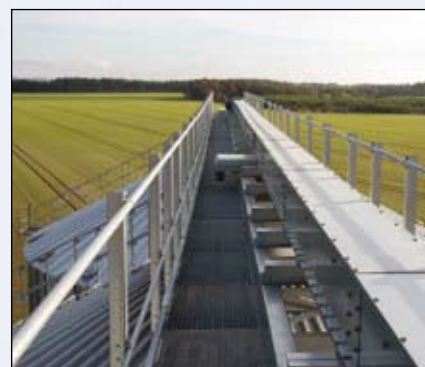
Kongskilde KCC chain conveyors - for horizontal conveying with great importance attached to high capacity and low energy consumption.
