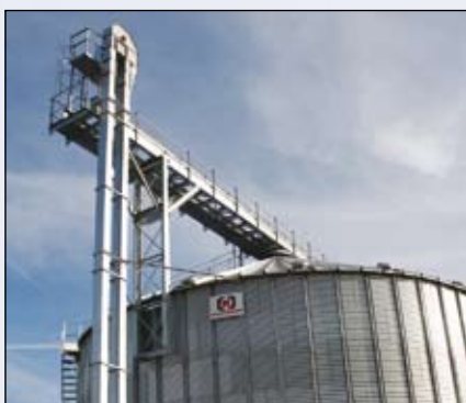
Kongskilde KBE bucket elevators - gentle vertical conveyance with low energy consumption.
