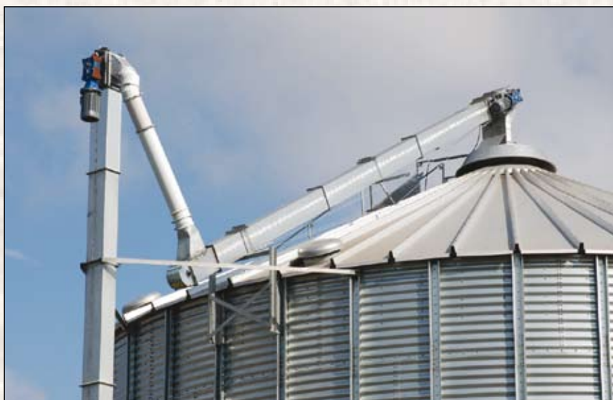
Horizontal, vertical and inclined conveying is possible with a CFG chain elevator.
